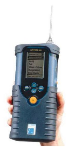
Single Class classification can save training time by allowing the identification of an unknown component without requiring the Cyranose 320 to be trained against other possible components.
